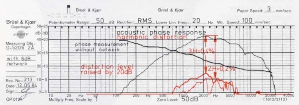
The acoustically measured phase runs as a straight line from 100 to 20.000 Hz.
