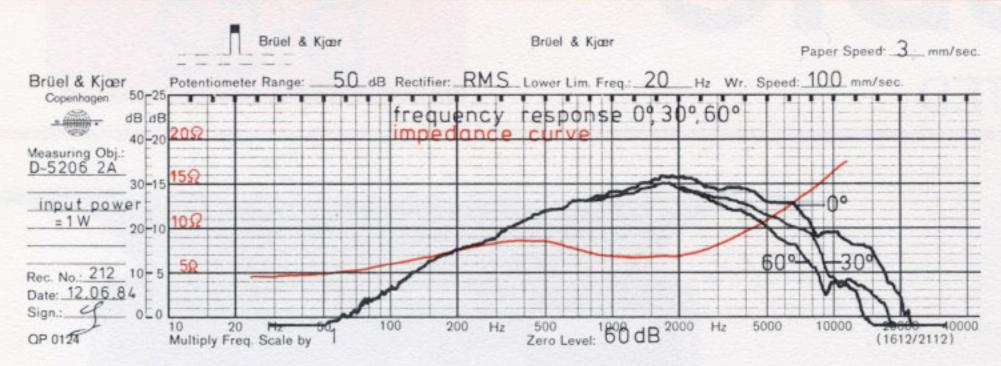
The dome shape of the frequency response curve is ideal for a midrange driver as with 6 dB filters the results come out perfectly.
