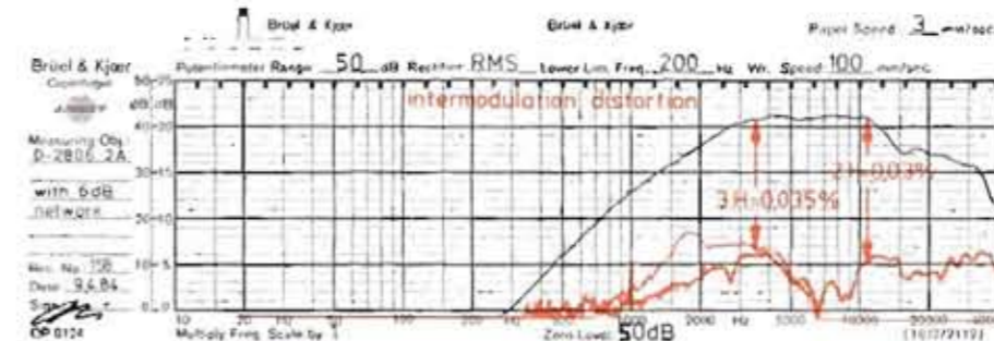
What other system has data like these? Intermodulation distortion level had to be raised by 40 dB.
